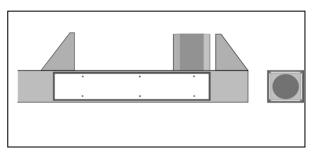
mechanical slide system that clamps around the edge of the steel I-beam. As this steel-on-steel slide system wears, it sharpens the edge of the I-beam to the point that it can be very sharp to work around. These systems quickly wear out needing far more maintenance.
